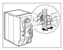
Remove the power supply cable and the drain hose from the hose holders. 8.
